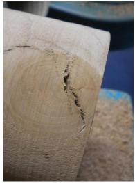
You might notice in the above photo a crack had appeared in the centre of a large knot and a few smaller ones around the knot. A wise man might have abandoned the whole thing at this point, but not me. It was another candidate for making a filler with sanding dust and glue. Eventually though, I cut the whole nasty thing off because I had made the hole for the mortar too deep anyway!
