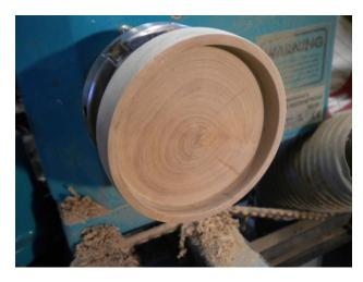
Here is the lid once I had hollowed it out, with the recess almost the right size to fit on the shoulder of the base.
