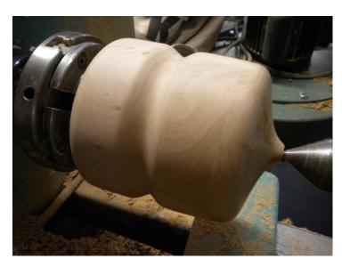
The lid fitted very nicely so that I could cut the two pieces together and cut away the tenon to give a little peak for mounting a knob. This photo does show the two pieces together honestly. The join does look pretty good doesn't it? Have you heard about pride and falls taking turns? Coming soon.
