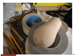
Here it is after some careful (for me) measuring to ensure the lid would fit around the correct place on the pear when stood in the base. I did it all between centres with a tiny link on each end which sanded away after cutting off.
