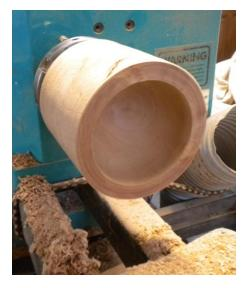
Here is the base with the outside smoothed off and petty well hollowed as much as I want for a mortar. I tried to get the hole hemispherical. Any round scraper would do this.
