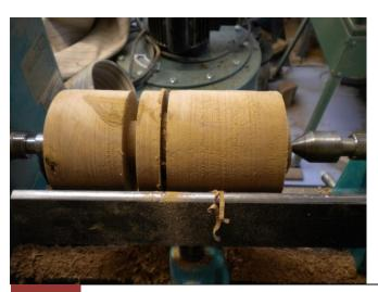
and another just avoiding the crack, and another thinner one to separate the lid from the base. The base is on the right, the lid in the middle of the picture here. The left hand end is mainly waste, though I might saw the crack off and try to use the rest.
