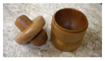
Here are the final three pieces, the pear and the inside bowl sunflower-oiled, ready to go together. The end grain soaks the oil in very quickly - you can watch it vanishing – so just keep oiling it until it doesn't.
