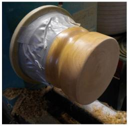
This picture shows the base mounted on a jam-chuck so that I could cut away the mounting tenon. You might notice the duct tape holding it securely. This needs to be <u>very</u> secure before you start sticking a chisel into the quickly spinning wood, or it will suddenly rip nastily and your lovingly crafted mortar will fly off around the room. I speak from experience.
