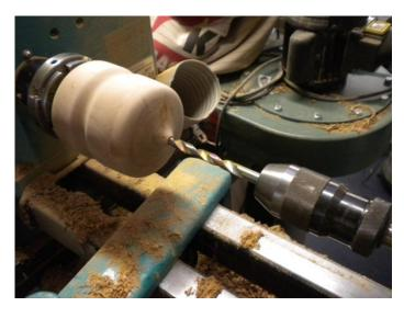
Here I am drilling out a 10 mm hole for the knob.
